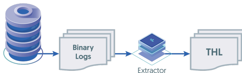
Figure 2.2. Internals: Cloud-Managed/Remote Database, Offboard Extraction
